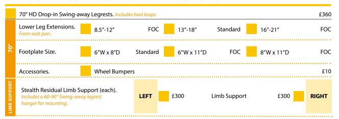
The 8"W footplates may cause interference with seat widths less than 19". Each limb support includes a 60-90° Swing-away leg support hanger for mounting.
